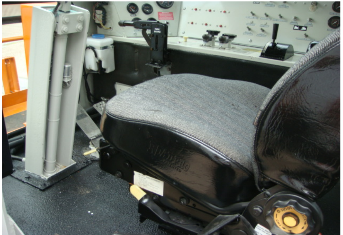
New 10 gauge steel overlay floor coated with two party polymer coating with abrasive to help prevent operating slipping. New windshield wiper squirt reservoir, motor/pump, and hosing
