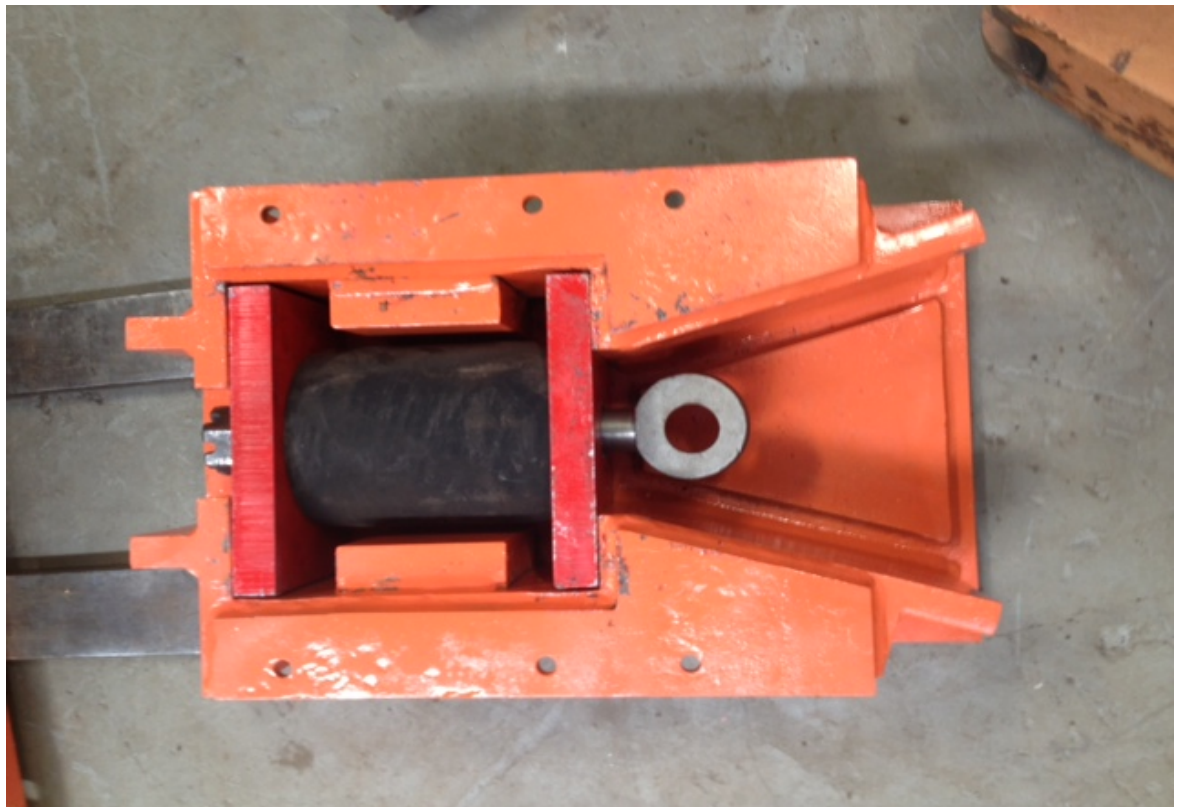
Photo shows the inside of the coupler receiver box during remanufacturing. New cushion block, new cushion block 1 inch end plated (red), new 18 inch drop forged eyebolt with new castellated nut. New coupler box to frame pin bushing.
