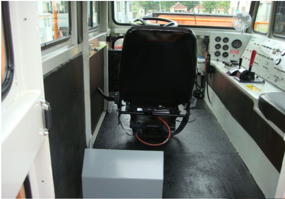
All new cab insulation, dome lights, air windshield wipers, and air horn valve. New steering wheel.
