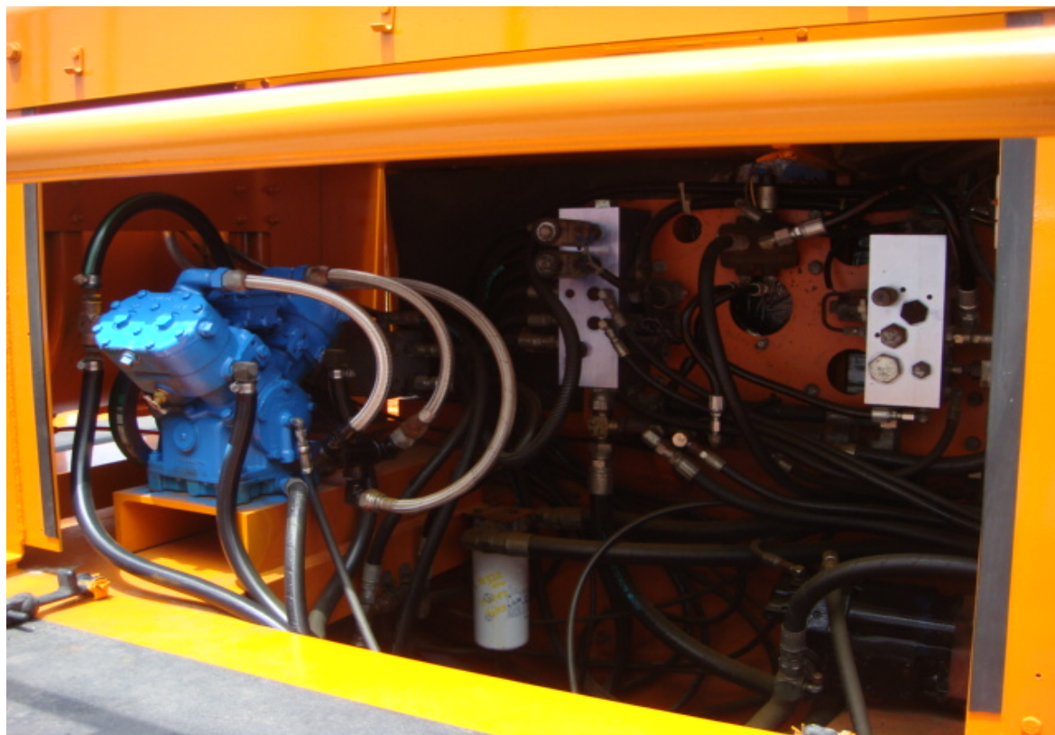
Remanufactured air compressor, compressor hydraulic motor, hydraulic pump
