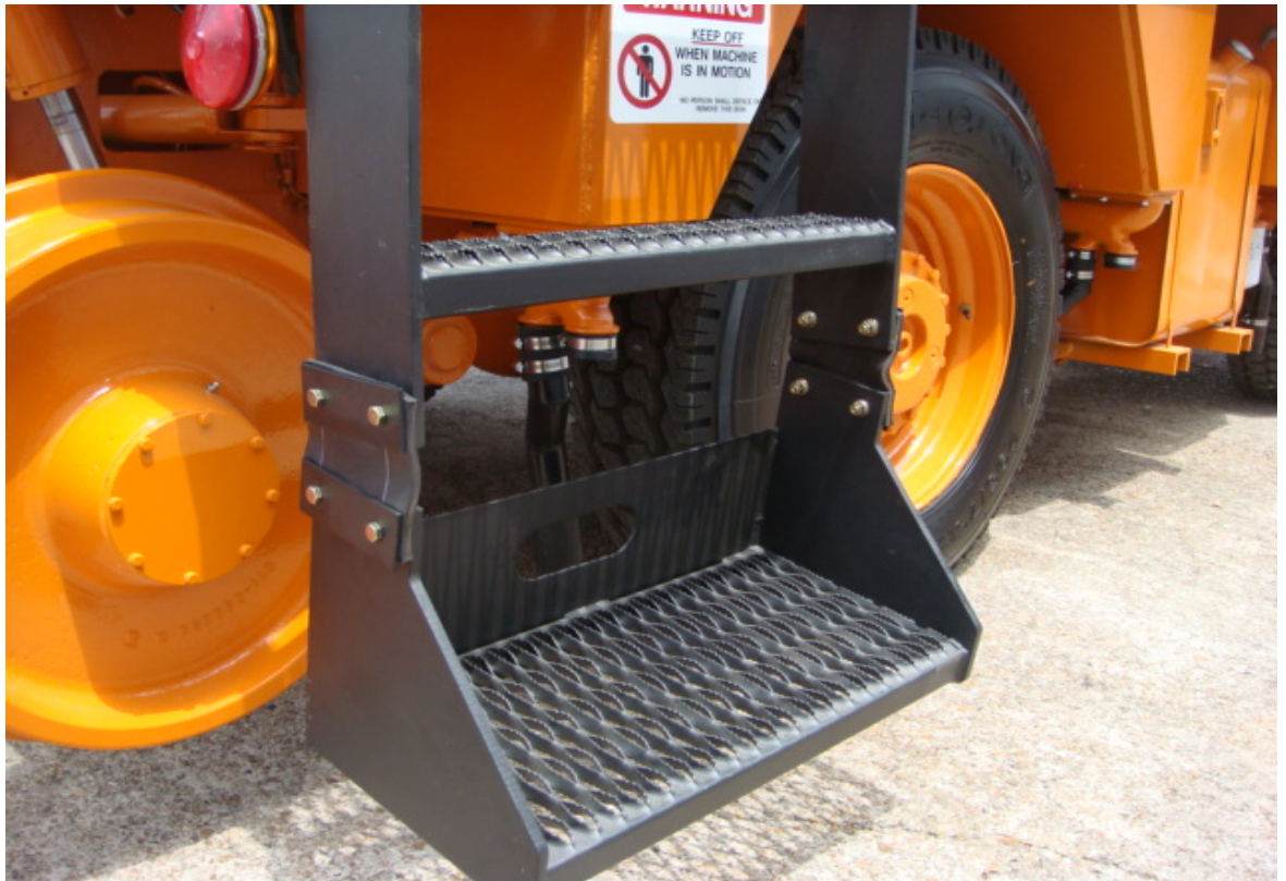
Powder coated ladders with break away first step
