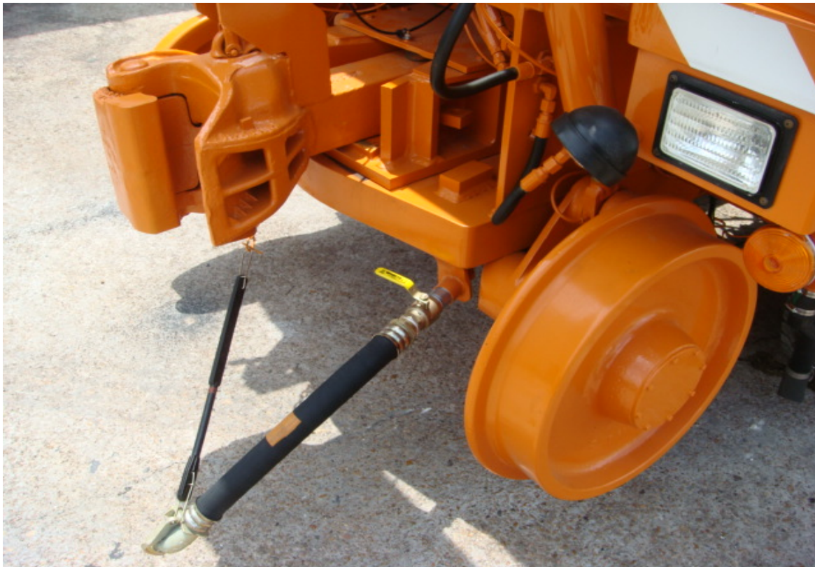
Photo shows rebuilt coupler, new rail lights, new angle cock, new train-air hose with gladhand and AAR bunji. Several rail wheels are new.
