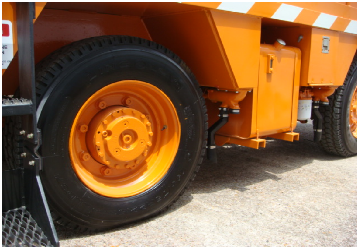
Hydraulic and fuel tank were removed and professionally flushed
