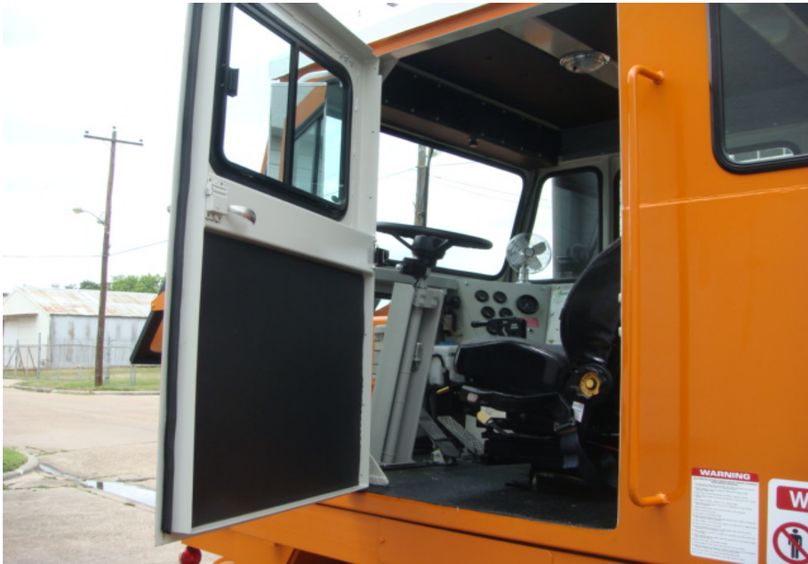
Photo show new operators door, hinge, handle, door check, coachman loops, one inch perforated vinyl insulation. New black anodized aluminum sliding door window.
