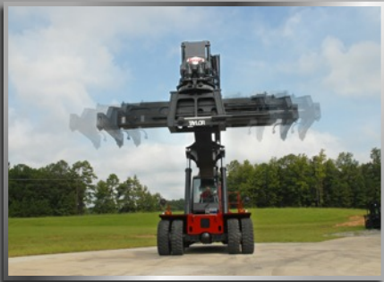
Hydraulic sideshift and mechanical pile slope. (Hydraulically powered pile slope and wide twistlock position available.)
