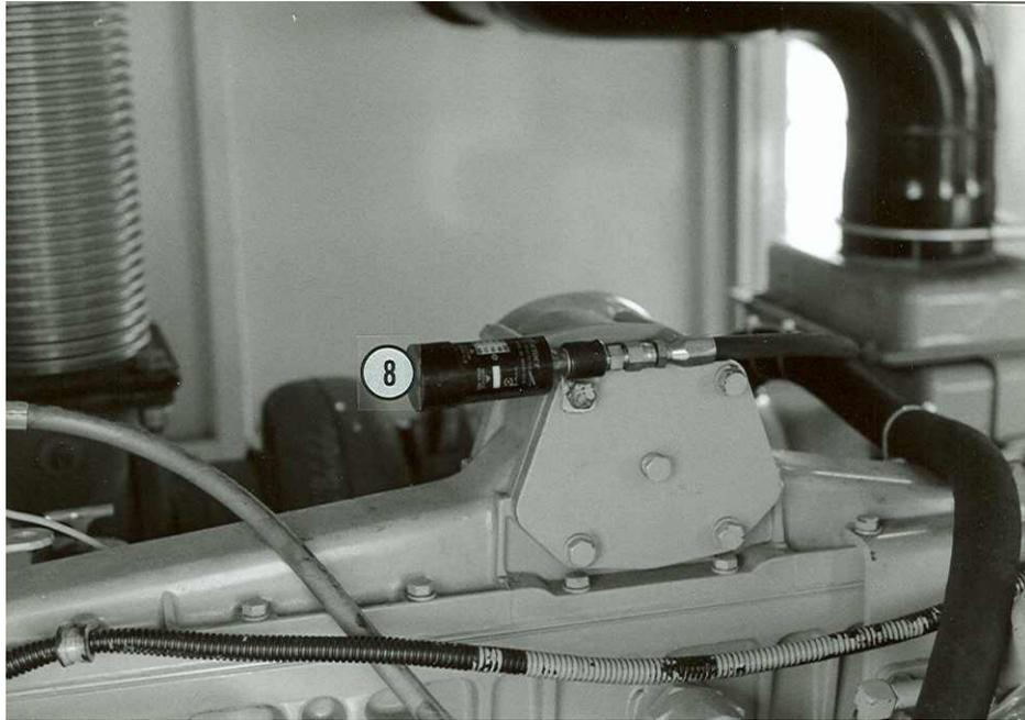
8. Air Cleaner Indicator- Mounted on the top of the engine is a vacuum indicator to show the condition of the engine intake air filter. As the air filter gets dirty the indicator will show more and more vacuum. With the engine shut down the indicator will remain at the highest reading until it has been reset by depressing the end of the indicator.
