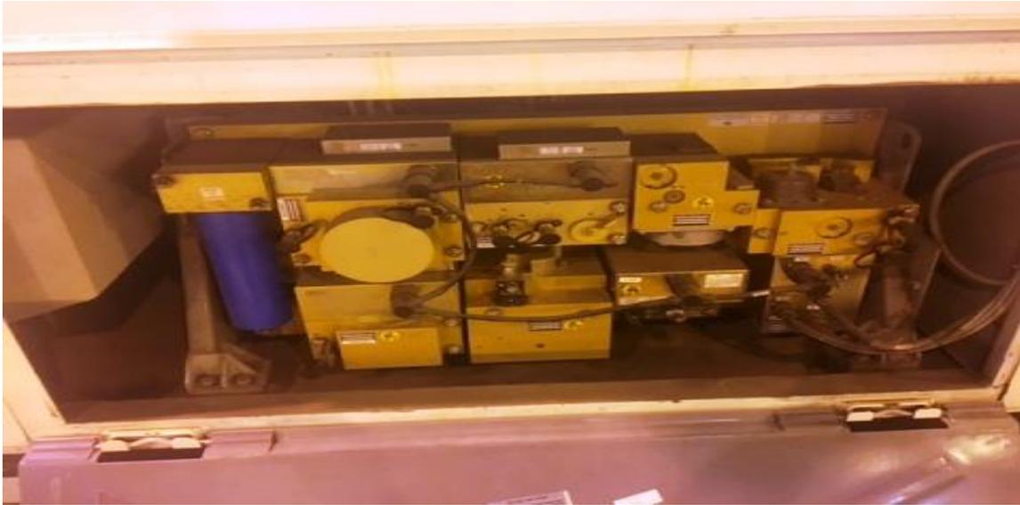
This is the CCB-26 lum rack for the air valves. This is the most modern air brake system developed by New York Air Brake.
