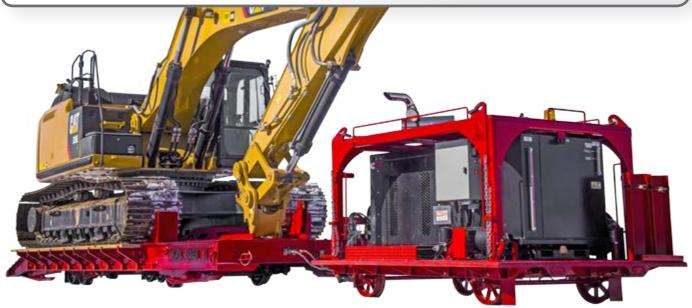
The heart of **The Dymax RailRider II** high rail system is the Power Car and the Machine Car. The Power Car features a Cummins engine with 240 horsepower.
