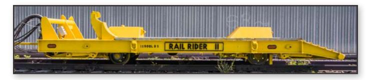
Dymax Rail Rider II Machine Cars are matched to the given excavator class for hauling capacity and lifting requirements. Machine Cars are available in end load designs. The end load design keeps the machine as close to within W6A load gauge as possible.
