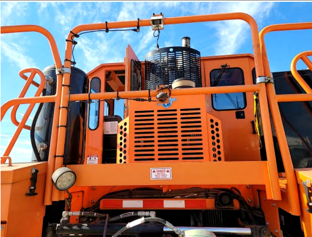
Intake Screen / Backup Camera / 09-27-2021
