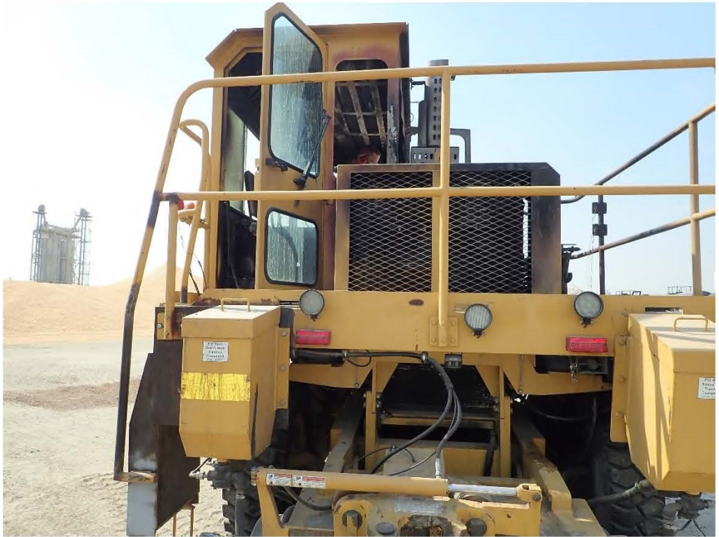
Photo No. 1: Rear of Titan Trackmobile; fire damage to cab
