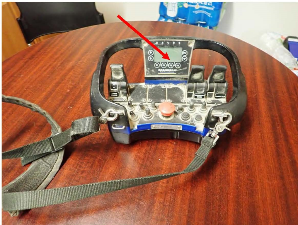
Photo No. 10: Scanreco radio remote control used on Trackmobile prior to fire
