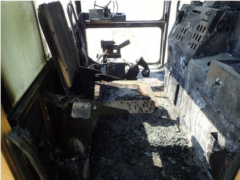
Photo No. 6: Fire damage to cab area of Trackmobile
