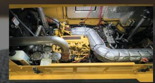
QSL-9 Liter Cummins Electronic Turbocharged Diesel Engine-Tier IV
