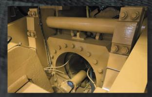
Heavy Duty Split Mainframe with Oscillating Bearing for Free Axle Pivot
