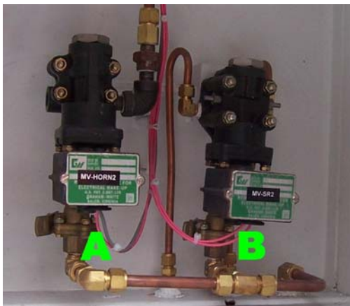
Fig. 2-28 – Rear Horn and Sander Magnet Valves
