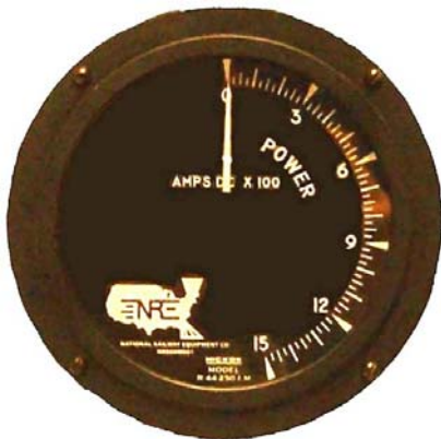
Figure 5-5 – Load Current Indicating Meter
