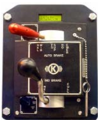
Figure 4-5 - Vertical (Bulkhead) EBV
