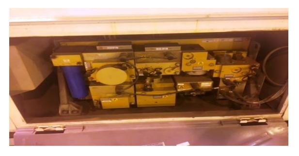
This is the CCB-26 lum rack for the air valves. This is the most modern air brake system developed by New York Air Brake.
