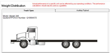
Recommended Payload Center of Gravity to achieve specified ground loads; measured from centerline of drive axles: 55 in. from the centerline of the drive axle(s).
